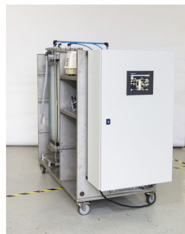
MABR System (Lab Scale OxyMem MABR front, back and side view)
