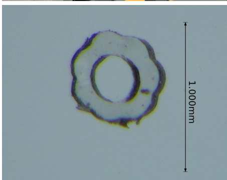
Hollow fibre membranes: bunches overview and singular membrane petal shape cross-section.
