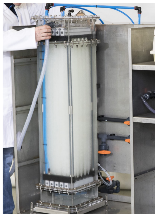
Oxyem Lab Scale MABR tank fitted with 5 mini cassettes
