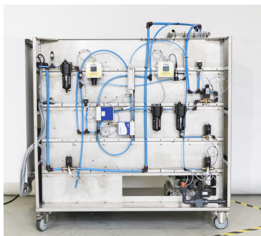
MABR System (Lab Scale OxyMem MABR front, back and side view)
